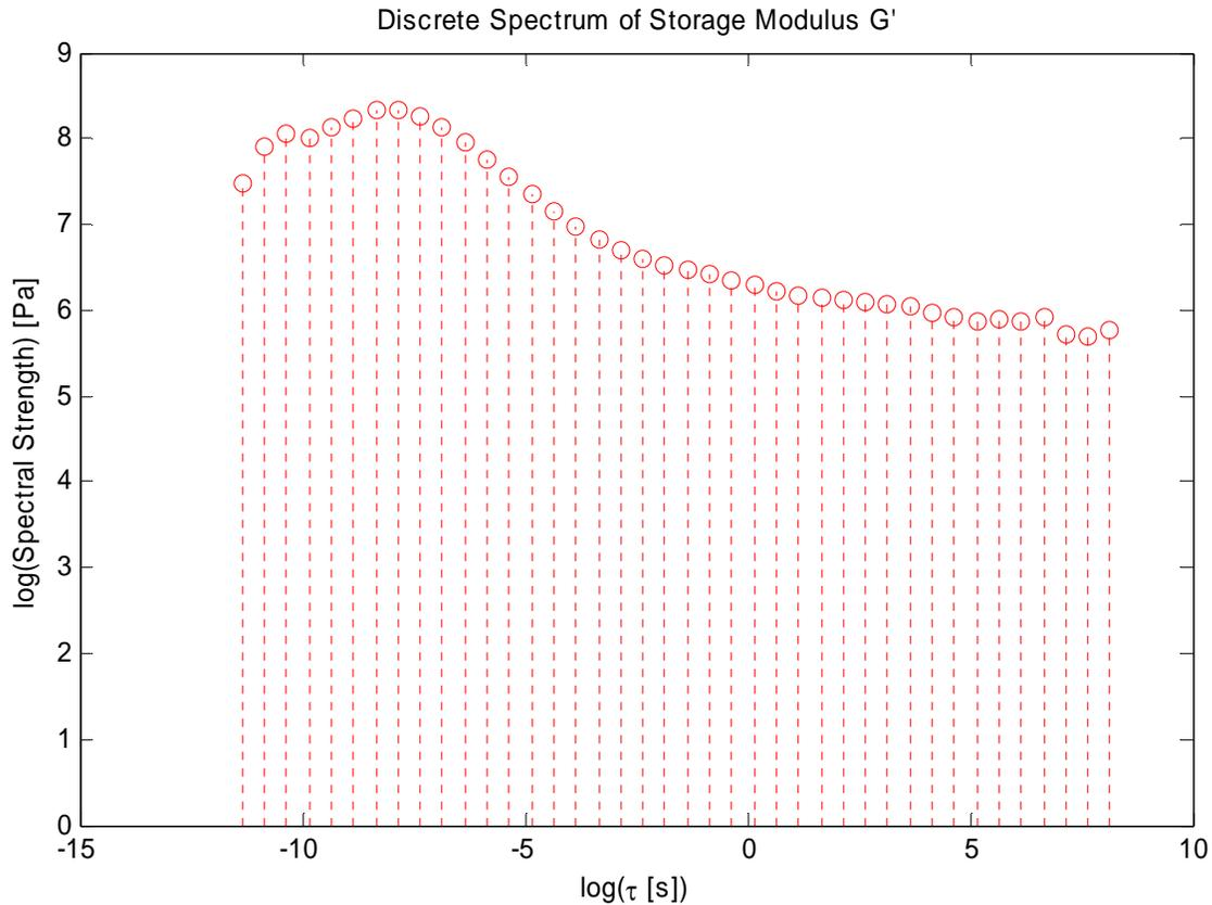
Figure 6. Discrete spectrum of the storage modulus  $G'$ .
