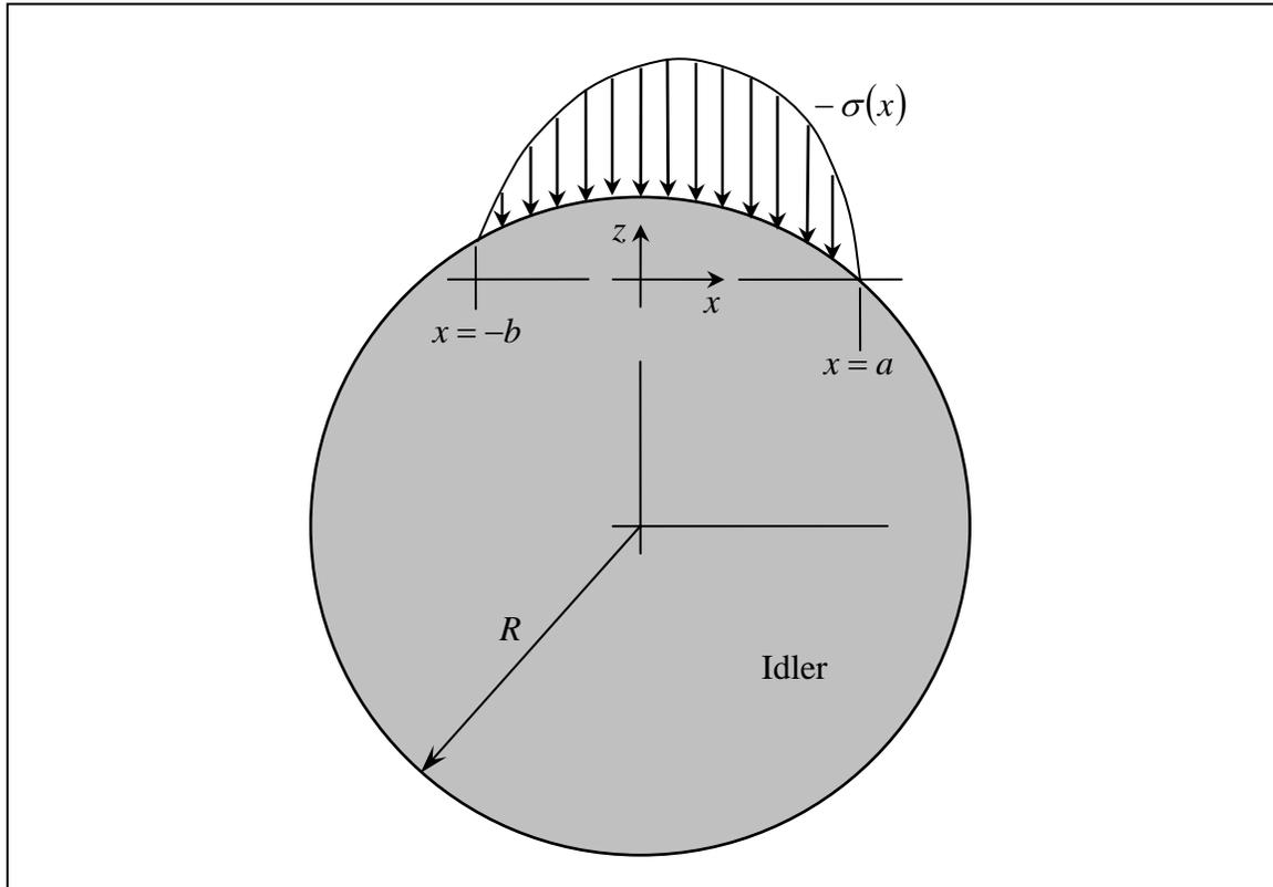
Figure 2. Contact stress distribution between idler and backing.
