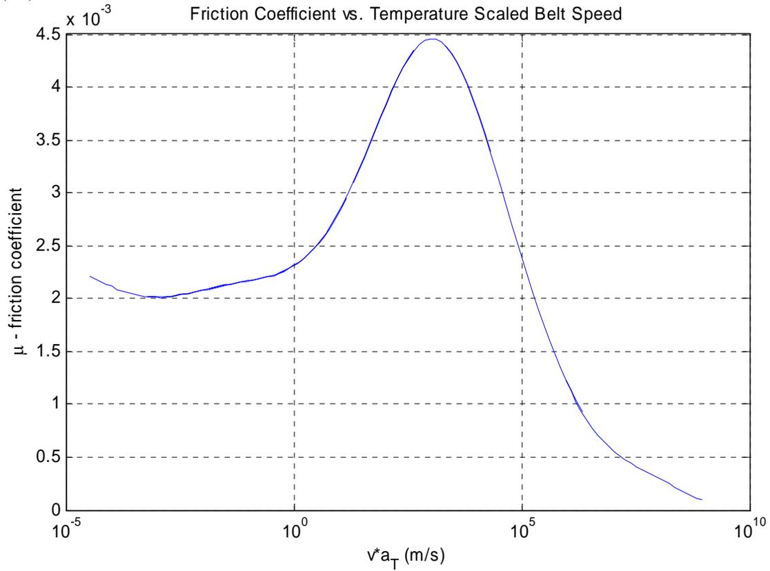
Figure 7: Indentation resistance  $\mu$  vs. scaled belt speed.
